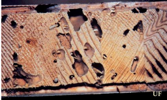
Fig 5. Drywood galleries that extend across the grain of the wood. Photo: R. H. Scheffrahn, UF.
